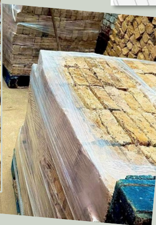
Site 2: A selection of the bricks and slates that have been hand-prepared for reuse
