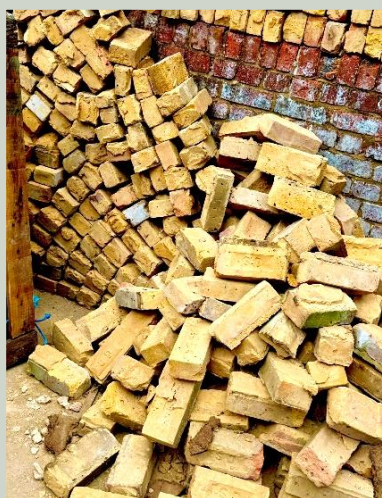
Site 2: A selection of the bricks and slates that have been hand-prepared for reuse
