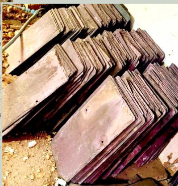
Site 2: A selection of the bricks and slates that have been hand-prepared for reuse
